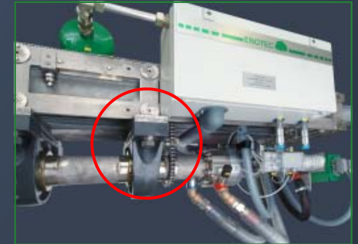
The CEMTEC® turning drive
