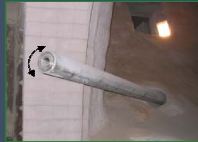
The turning CEMTEC® cooling protection tube inside the combustion chamber
