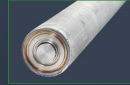
The top of the push plate inside the cooling protection tube
